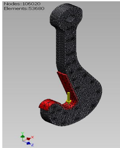
Fig.3 3-D Mesh Model of Laminated hook
